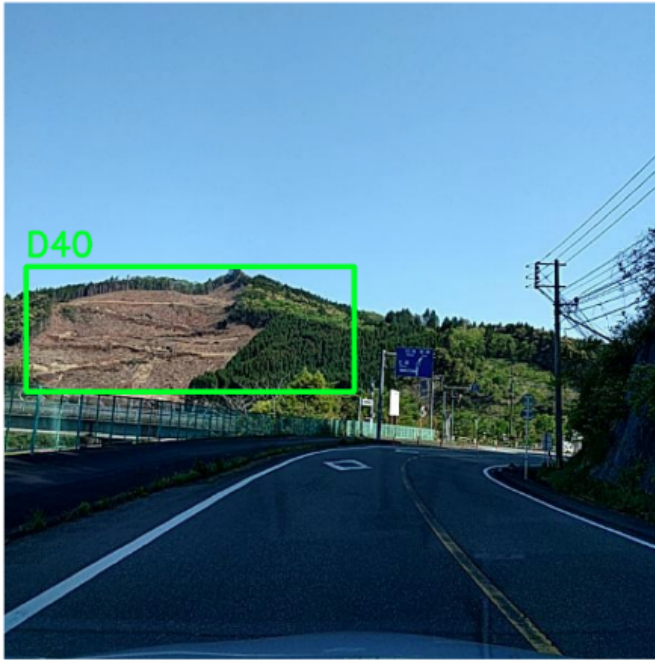
Fig. 9. An image ( Japan_002970 ) with wrong pothole damage bounding box in the training set for Japan. This mistake is obvious to humans and less clear to machine learning models. Thus, it might indicate that a machine learning model generates this label, and the error was slipped through the human quality check step.
